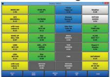
Hot start "Cart Wall" for on demand instant playback of beds, sound effects, ID's, feeds and any audio item in the library. Play or insert to current schedule. Color coded by category for quick recognition. Support for 4 discrete audio channels and up to 32 virtual audio channels with a dedicated meter in the header bar.
